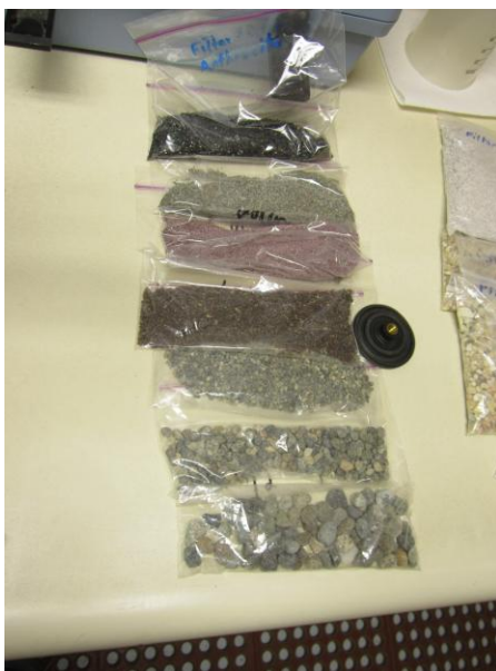
Final filter media – filter #4
