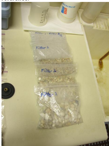
Clarifier media – pre filter #2
